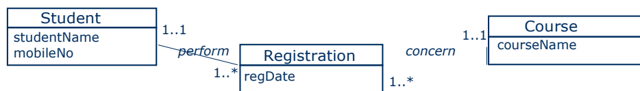
Figure 1. Conceptual model of a small domain in UML.
