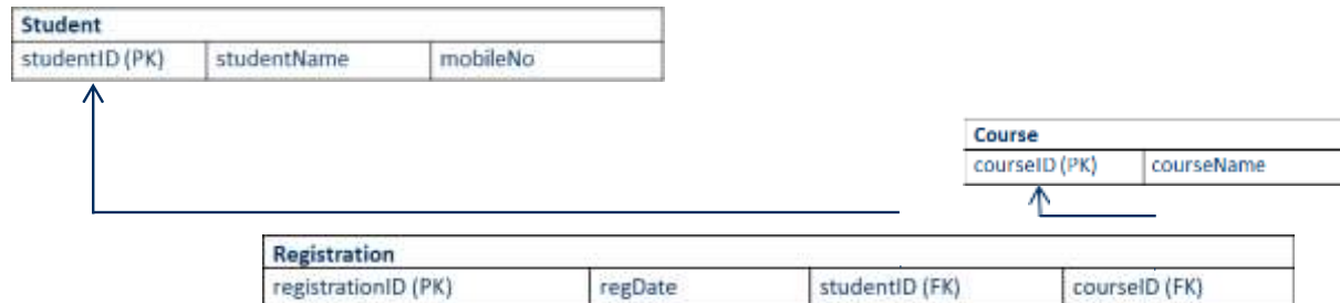
Figure 3. Relational Database Schema in form of columns of tables
