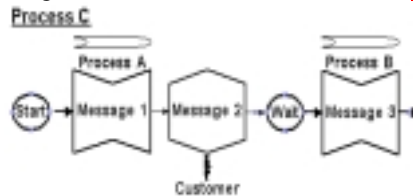
Fig. 4. The BML diagram visualizes the order in which the messages shall be sent and received in a process. Note that the figure only shows the beginning of a Process.
