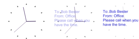
Figure 5: The iClock, first showing the time and then fading in a message for one of the participants in the room.
