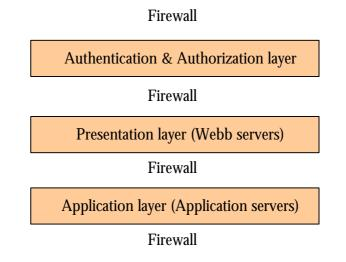
Figure 1. Firewall architecture.
