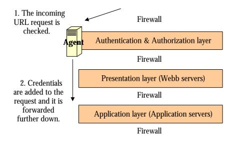
Figure 2. Description of how the SiteMinder security product for securing webb applications work.
