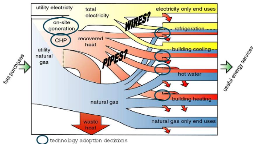
**Figure 1. Typical Sankey Diagram (Marnay *et al.*, 2008)**
