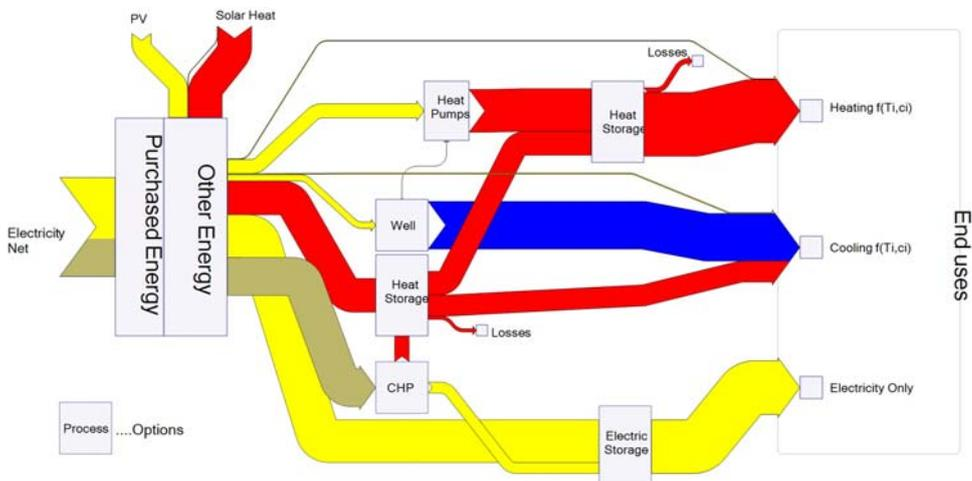
**Figure 12. Alternative System Configuration for ENERGYbase with CHP and Storage**
