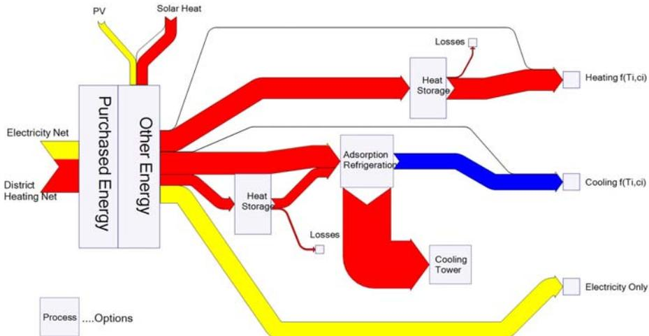
**Figure 10. Alternative System Configuration for ENERGYbase with District Heating, Heat Storage, and an Adsorption Chiller**
