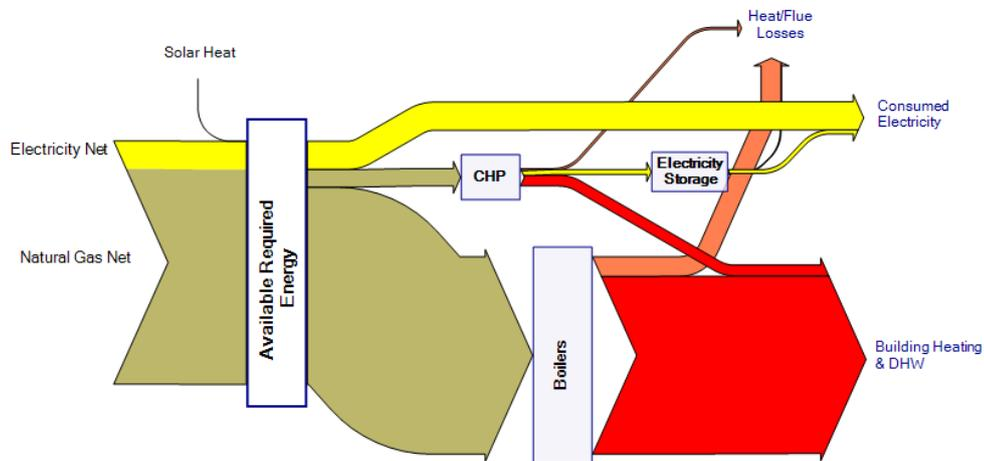
**Figure 9. Alternative System Configuration for FASAD with Electricity Storage**
