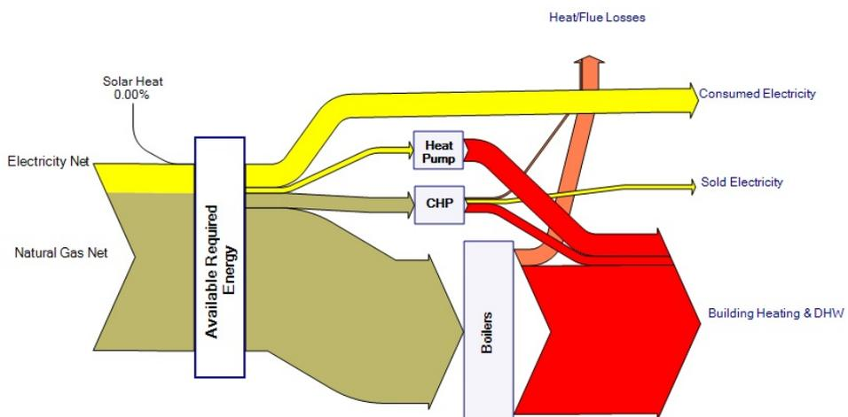
**Figure 7. Alternative System Configuration for FASAD with Heat Pump**
