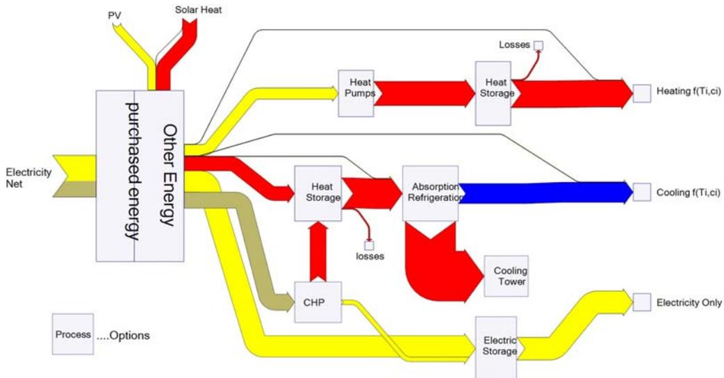
**Figure 11. Alternative System Configuration for ENERGYbase with CHP, Electricity and Heat Storage, and an Absorption Chiller**
