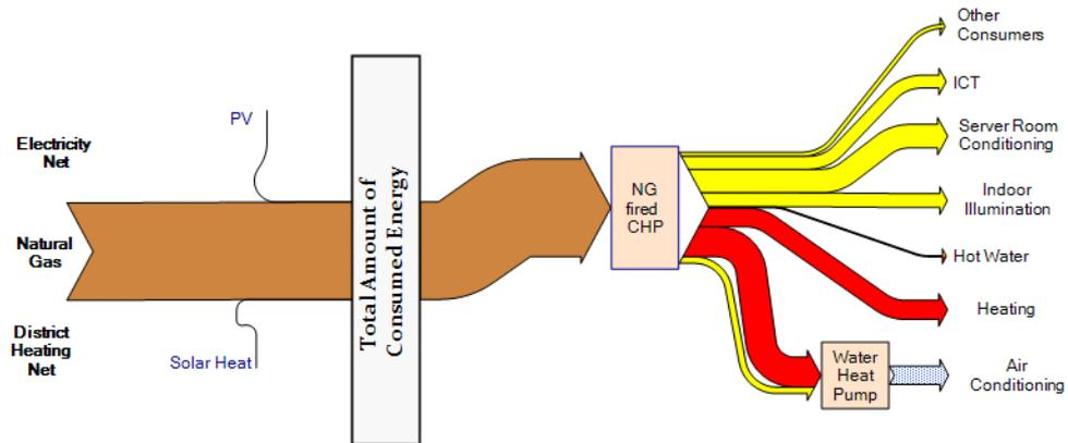
**Figure 5. Alternative System Configuration for Pinkafeld with CHP**
