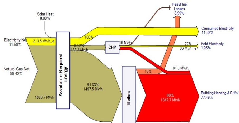
**Figure 3. Sankey Diagram for FASAD**
