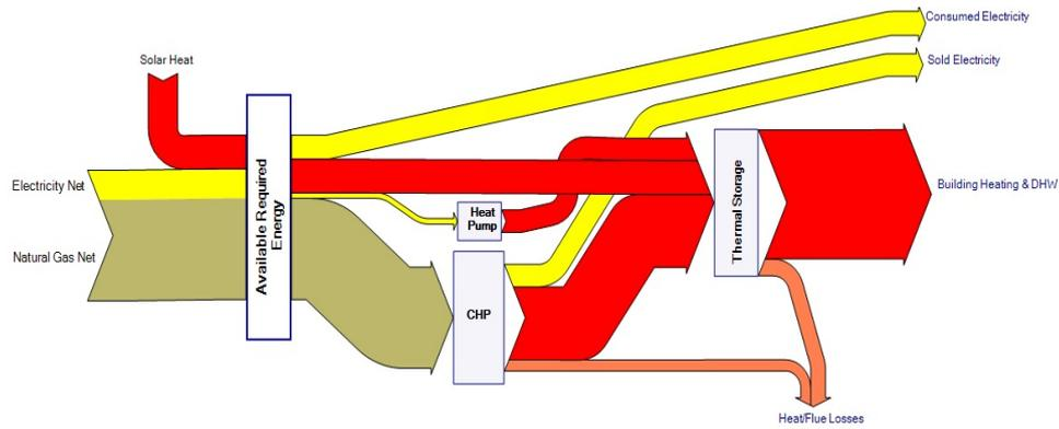
**Figure 8. Alternative System Configuration for FASAD with Solar Thermal System and a Large CHP System**
