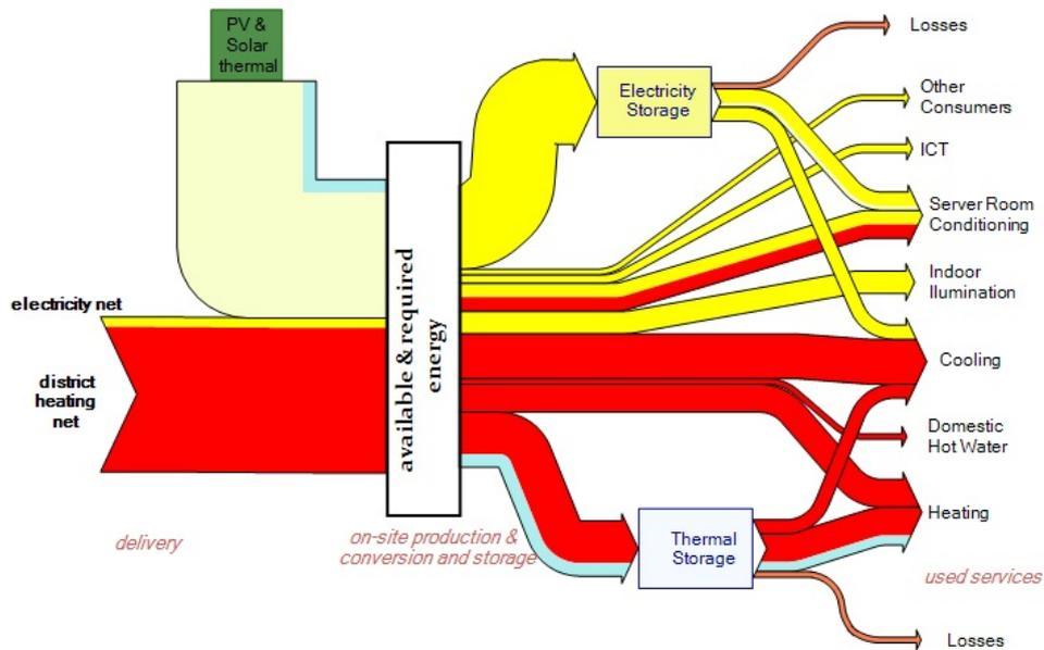
**Figure 6. Alternative System Configuration for Pinkafeld with Storage**
