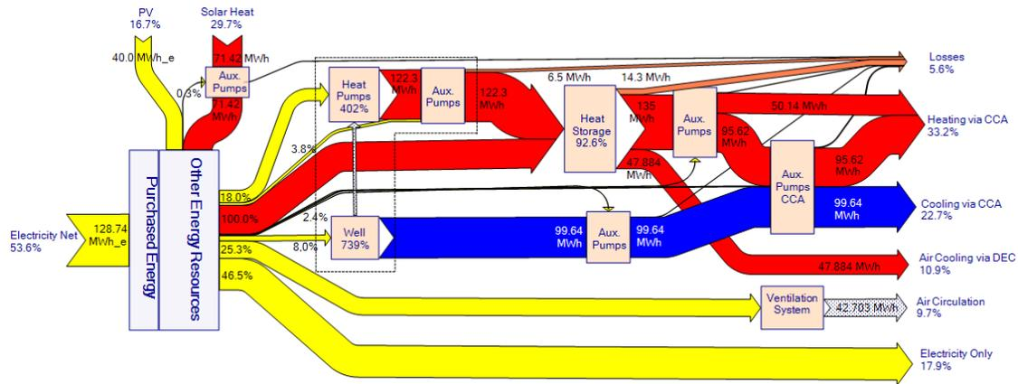
Figure 4. Sankey Diagram for ENERGYbase
